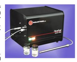
distillation temperature. They can also measure concentrations of species such as methanol or esters, and monitor transesterification reactions. The new product has improved sensitivity over previous analyzers, which has expanded the measurements that LT-NIR can perform.
